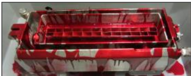
Fig. 1 Part of an encapsulation system: considerable criticality due to the assembly of the parts into a single body, which cannot be disassembled for the treatment.
